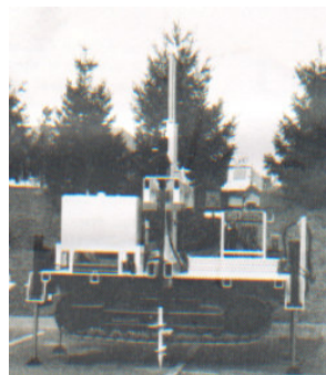
20 Ton Medium Weight CPT Crawler With Automatic Anchoring
